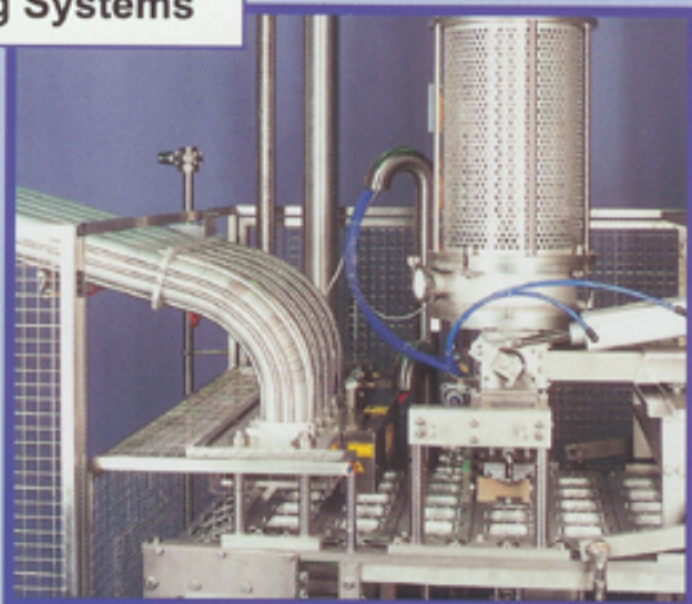
Special dosing system with compensation cylinder for petfood
